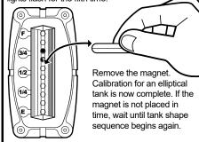
If the magnet is not placed in front of the display to select a tank shape, the tank selection sequence will continue and the FULL light will flash 5 times. After the FULL light flashes 5 times the tank shape selection sequence will begin again. (Step 5) The tank shape selection is made in this time, the display will default to a rectangular tank.
